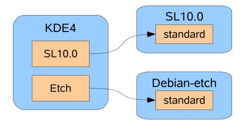
Packages will be built for both SL10.0 and Debian-etch. Each repository can also support multiple architectures.
